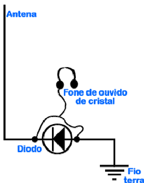
Figura 2.9 Receptor AM Simples
